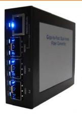
between 1000Base-FX fiber/ fiber and fiber to 10/100/1000Base RJ-45. RT-3600 equipped with a FX fiber port is a pluggable capable of supporting. Custom-made solutions are available; any **mini GBIC SFP LC** Transceiver (Gigabit: 550m to 70Km, Fast: 2Km to 120Km) is allowed to be chosen per your request.
